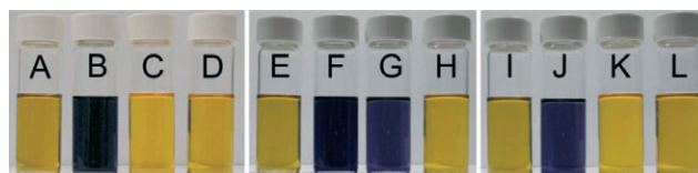
Figure 7. Color changes of 1 , 2a , and 2b (0.005 mM) upon the addition of 10000 equiv of 1°, 2°, and 3° amines in \text{CHCl}_3 : A) 1 only; B) 1 + 1° amine; C) 1 + 2° amine; D) 1 + 3° amine; E) 2a only; F) 2a + 1° amine; G) 2a + 2° amine; H) 2a + 3° amine; I) 2b only; J) 2b + 1° amine; K) 2b + 2° amine; L) 2b + 3° amine.
